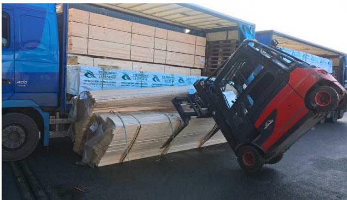
The forklift truck driver has not taken into account the weight of the batch of timber.
