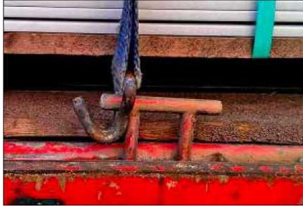
Do not attach the hooks at the end.
