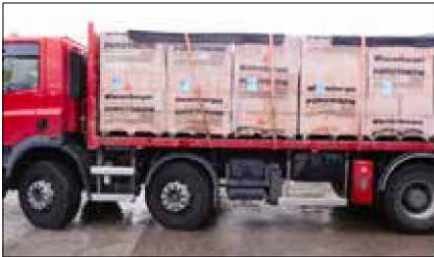
The straps placed must be tightened perfectly vertically.
