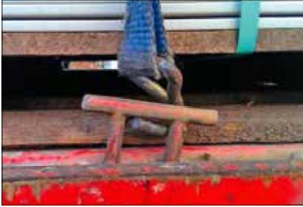
Chassis hooks must be correctly placed on the edge of the truck.
